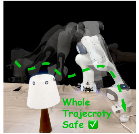
(f) Teleoperating near a lamp: positive clearance from obstacle preserved.
