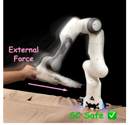
(c) With a UMI gripper, the arm cannot be pushed beyond the viability boundary.
