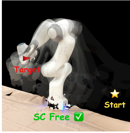
(b) With SCA enabled, the arm safely avoids self collision and reaches the target.
